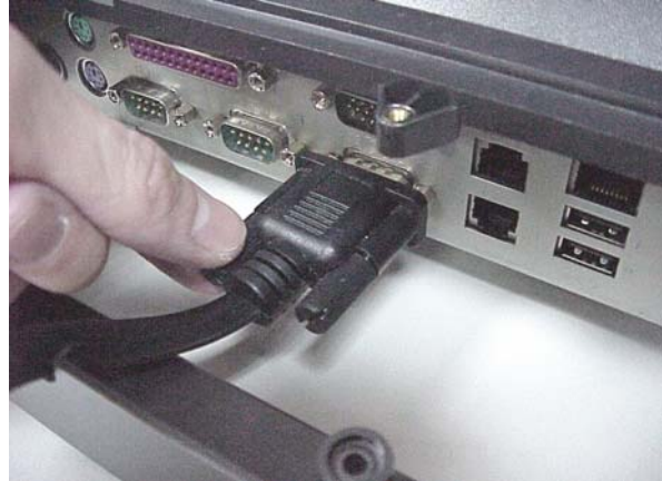
b. Fasten the two screws of the RS232 connector.
