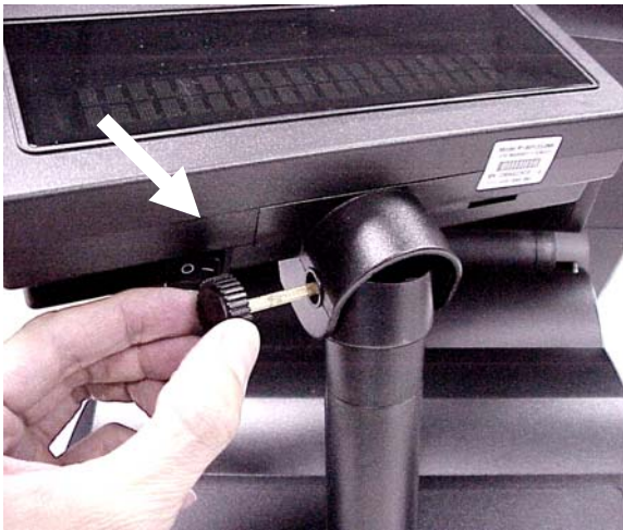
g. Insert the screw into the hole of the connection kit. Notice the direction of insertion.
