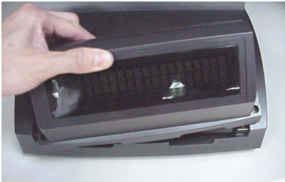
c. Connect the RJ45 before mounting the customer display.
