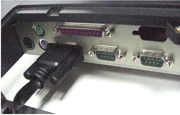
a. Connect the DB-9F cable to any of the COM ports.
