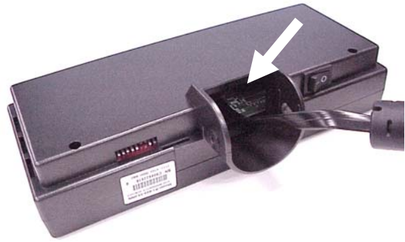
f. Insert the RJ45 connector into the jack of the customer display.
