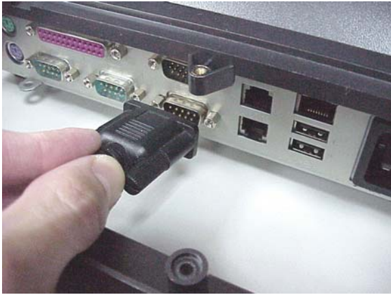
a. Connect the RS232 connector to any of the COM ports.
