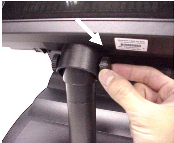
h. Fasten the cap at the other end of the screw. The installation is completed.
